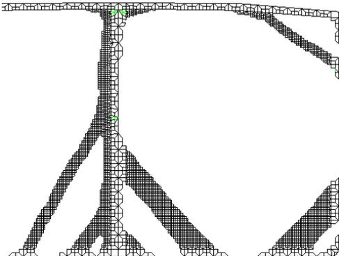
Fig.9 Typical topological configuration of web frame based on BESO method
