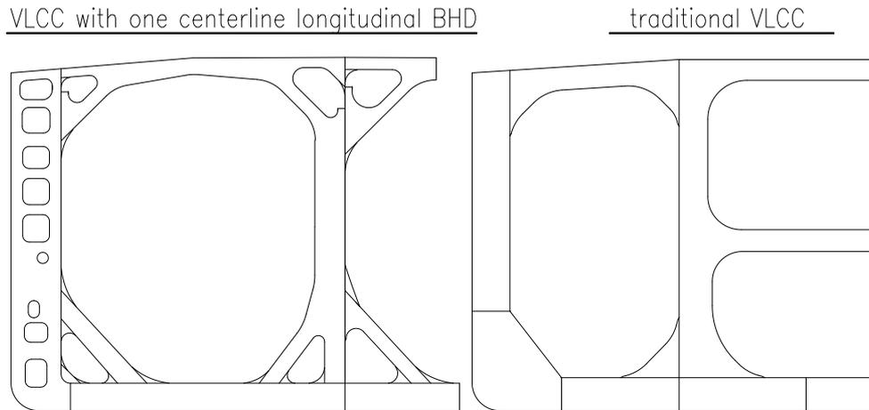
Fig.11 Comparison of typical web outlines between traditional VLCC
