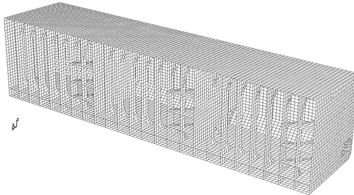
Fig. 4 Typical 3-Cargo Hold Models within Midship Region of Oil Tankers
