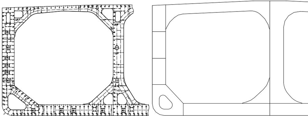
Fig.13 Comparison of typical web frame between Aframax oil tanker developed based on topology optimization and traditional Aframax oil tanker
