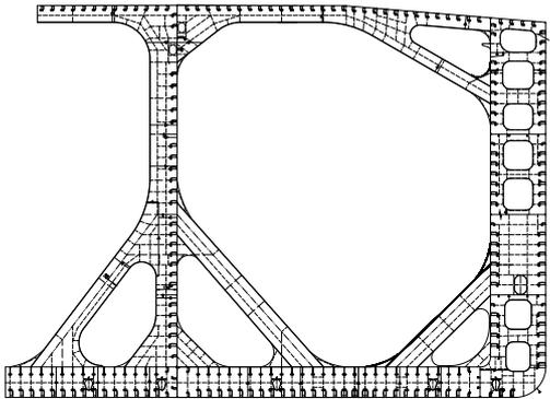
Fig.10 Drawing of typical topology optimal of web frame based on BESO method
