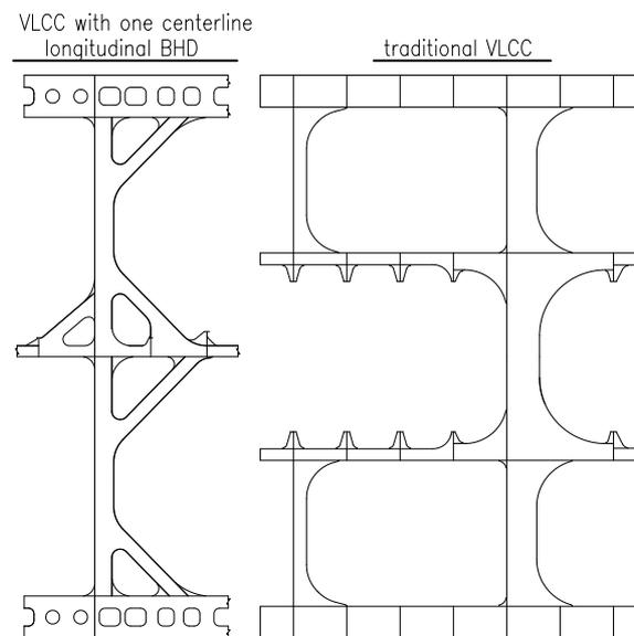
Fig.12 Comparison of typical horizontal stringer outlines between traditional VLCC
