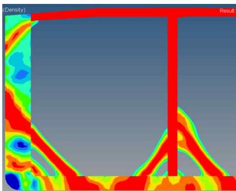
Fig.5 Typical topological configuration of web frame based on SIMP method
