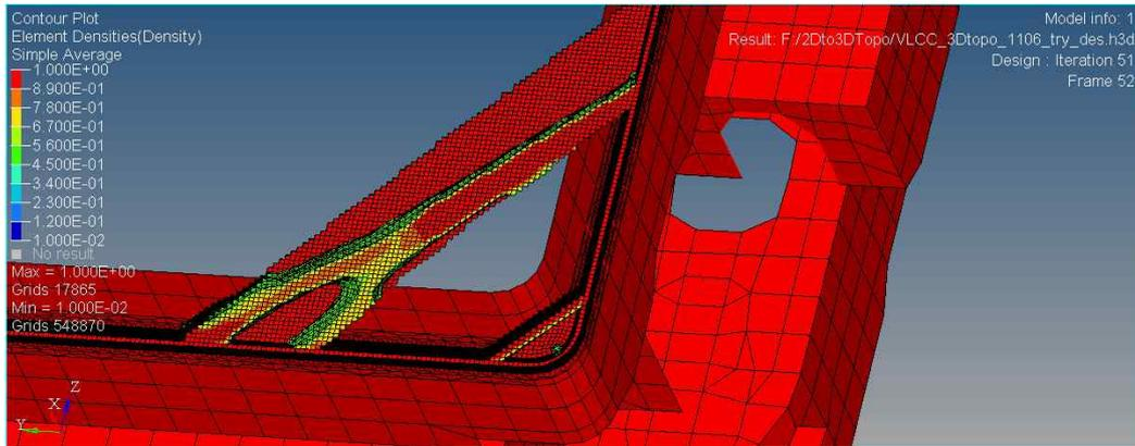
Fig.14 topological configuration of mixed shell elements and solid elements
