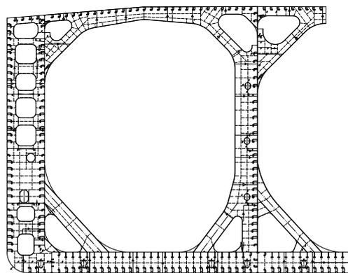
Fig.6 Drawing of typical topology optimal of web frame based on SIMP method
