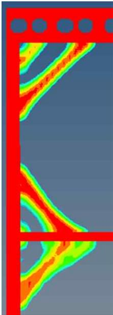
Fig.7 Typical topological configuration of horizontal stringer based on SIMP method
