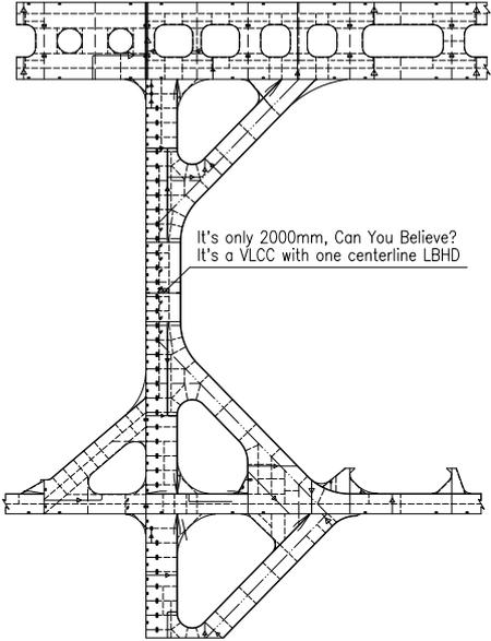
Fig.8 Drawing of typical topology optimal of horizontal stringer based on SIMP method
